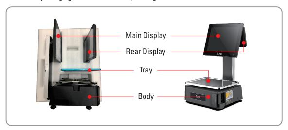
2. Remove the cover from the Main Display and connect it as shown below.
