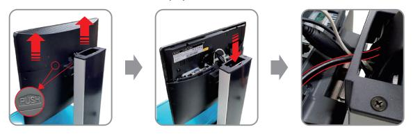
Route the cables on the Rear Display through the holes of the Pole Cover.
