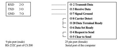
(2) COM2 - RXD: Pin No. 2, TXD: Pin No. 3, GND: Pin No. 7 (Option)
