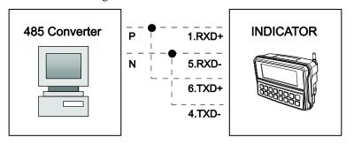
Note. RS-422 & 485 communication is optional specifications, which are supported through COM2. Refer to page 42 (Set Mode) for the setup.
